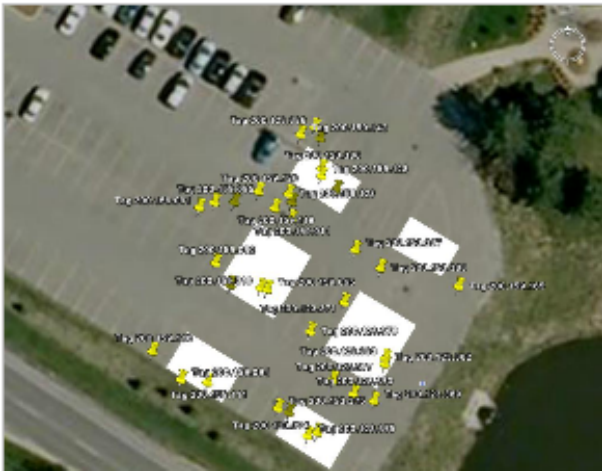
Figure 5. Tags Location on the Parking Lot of the University of Waterloo. Tags Are Deployed into the White Squares called here blocks. Yellow Points Represent Tag Location as Measured by a GPS.
